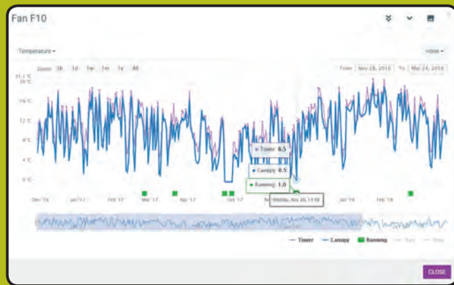
Showing the canopy temperature for each fan on the map as well as controller status, battery voltage, engine RPM, inversion temperature, ambient wind speed and fan running time for each fan.
